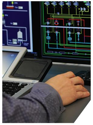
A Building Management System (BMS) is a computer-based control system installed in buildings which controls and monitors the building's mechanical and electrical equipment such as ventilation, lighting, power systems, fire systems and security systems.
